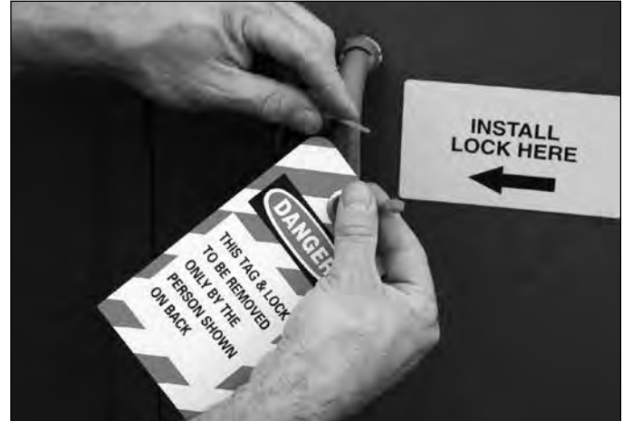
Turn off power, lock controls and tag
