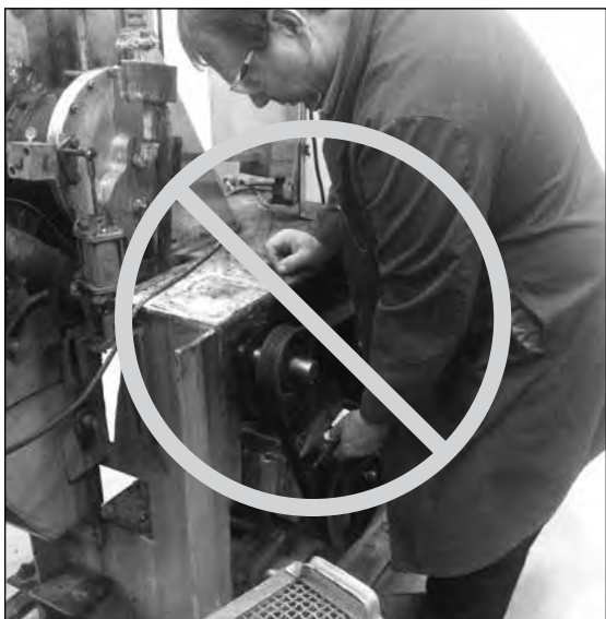
No loose or bulky clothing. This technician's bulky lab coat is a hazard near moving components
