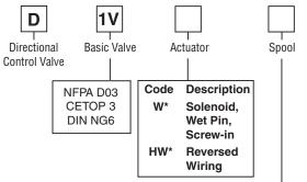
\* Valve schematic symbols are per NFPA/ANSI standards, providing flow P to A when energizing solenoid A. Note operators reverse sides for #008 and #009 spools. See installation information for details. To configure per DIN standards (A coil over A port, B coil over B port) code valves as D1VHW\*\*\*.
